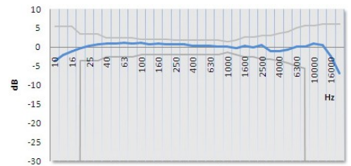
Free field response with Z weighting
